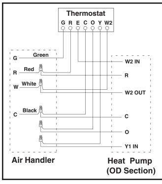
Figure 4. Typical Thermostat Connections
