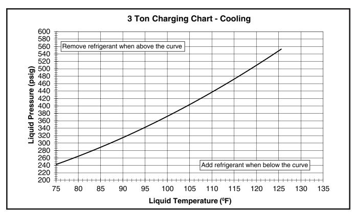
Figure 9. Charging Chart for 3 Ton Models (TXV Matches)
