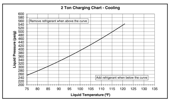
Figure 7. Charging Chart for 2 Ton Models (TXV Matches)
