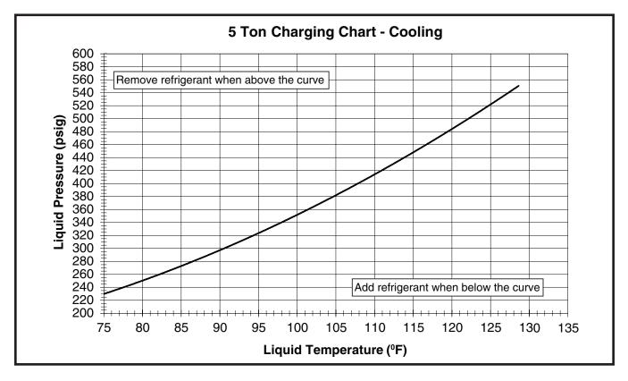
Figure 12. Charging Chart for 5 Ton Models (TXV Matches)
