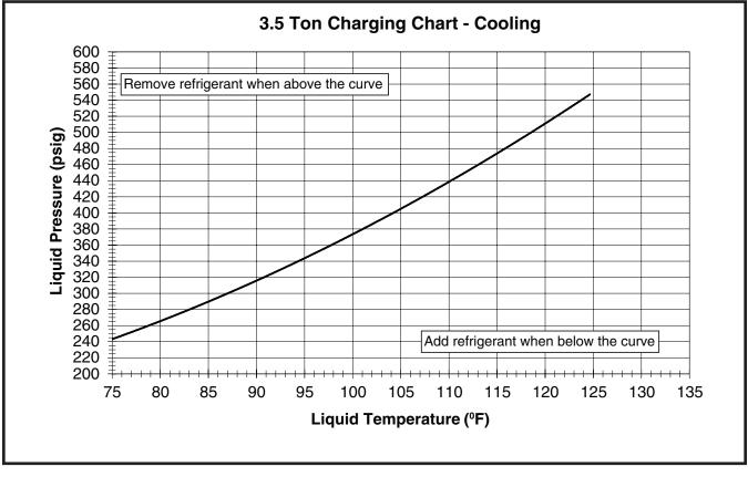
Figure 10. Charging Chart for 3.5 Ton Models (TXV Matches)
