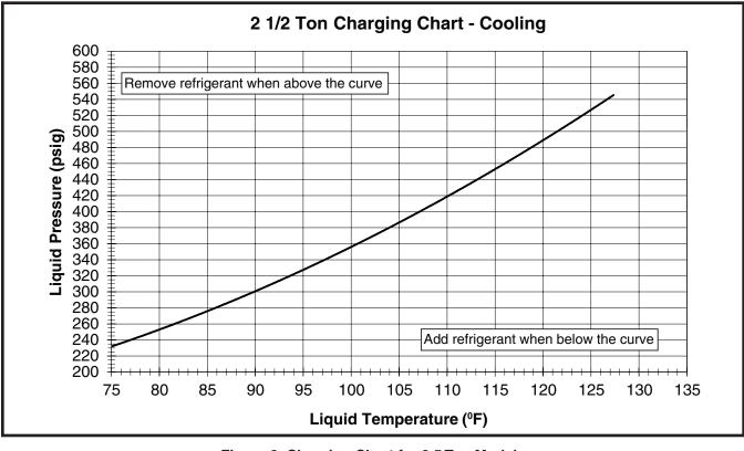
Figure 8. Charging Chart for 2.5 Ton Models (TXV Matches)
