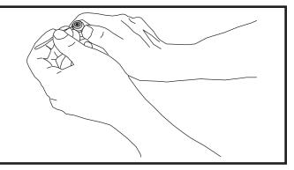
Figure 3. Removal of Orifice
