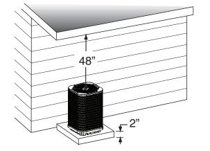
Figure 1. Clearance Requirements
