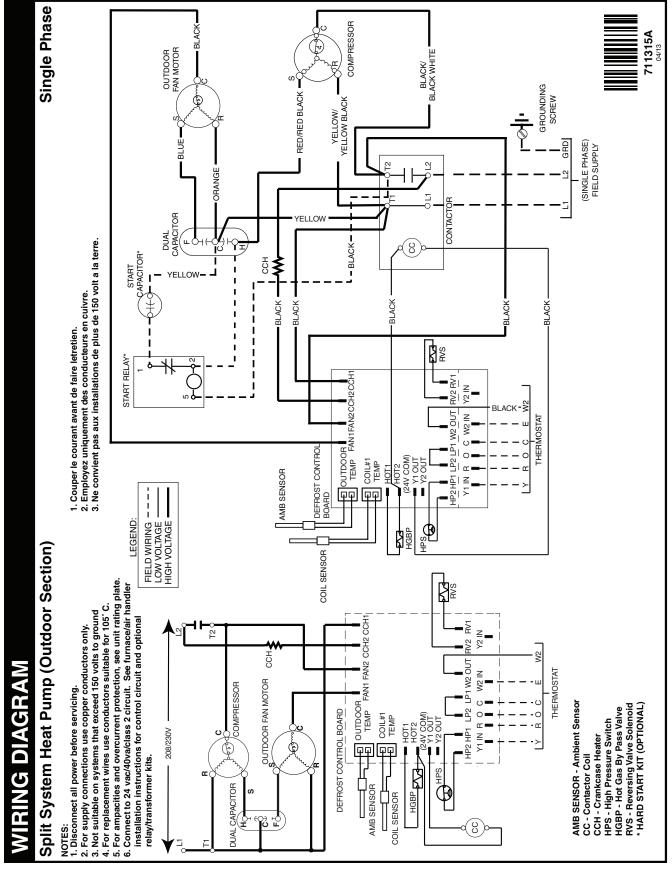
Figure 14. W.D. for 1.5 - 5 Ton Models NOT Equipped With CoreSense™ Diagnostic Module
