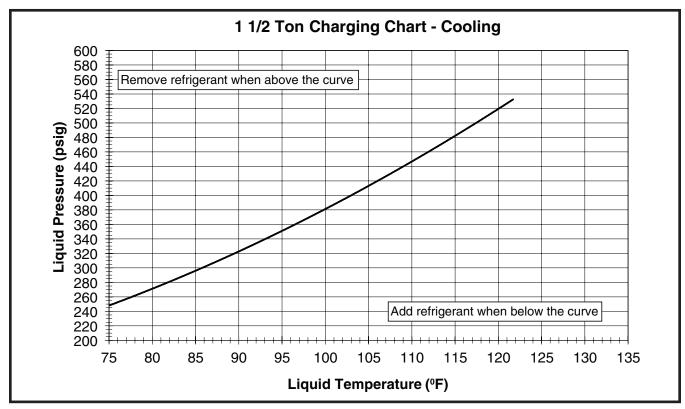
Figure 6. Charging Chart for 1.5 Ton Models (TXV Matches)
